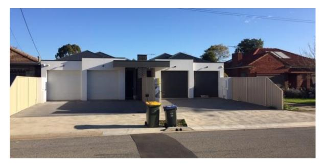
In this example in Henley Beach South, a double garage, with single width crossover and splayed driveway, allows for the same undercover car storage capacity as the above example, while retaining the existing street tree and soft landscape on the verge streetscape.
