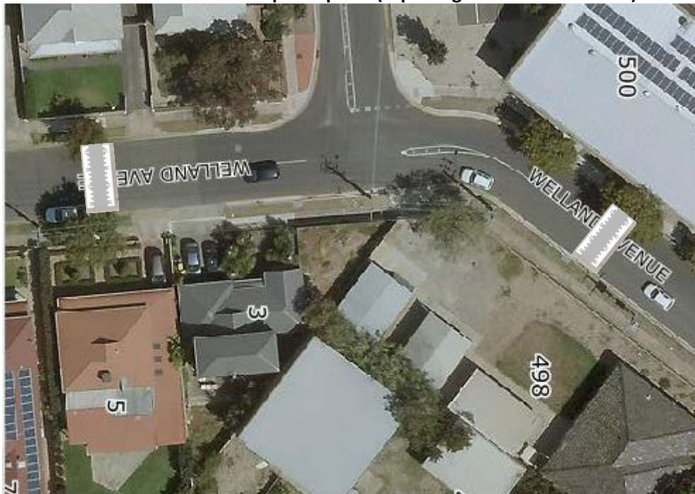
New Welland Avenue Road Humps Proposal (replacing Raised Intersection)
