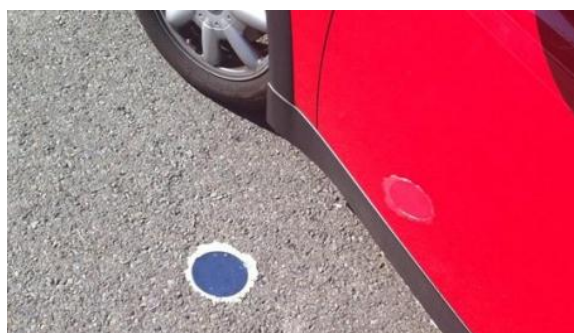
Figure 14: The circular sensor that wirelessly detects the presence of a car has a five year battery and transmits real-time parking data that can be displayed.
