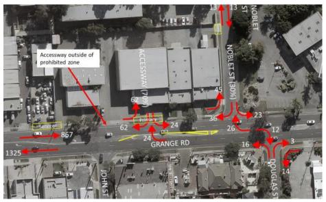
Figure 10: Option 2 – relocated accessway, all movements retained
