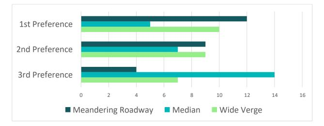
Based on the consultation results, we will be proceeding to detailed design with the Meandering Roadway option. As a result of feedback received, we will be including roundabouts at all 4-way intersections and incorporating additional Water Sensitive Urban Design (WSUD) elements into the landscaped area. We will be consulting further with residents on tree and understory species selection once the landscape design commences.
